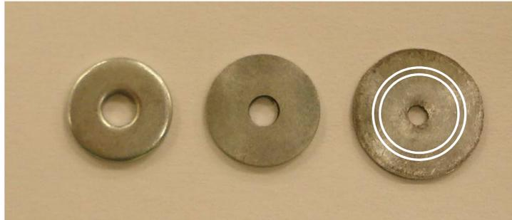
It has been shown that, when the ring length (thickness) equals the external to internal diameters difference, the traditional Kolsky expression for the material strength should be corrected to
